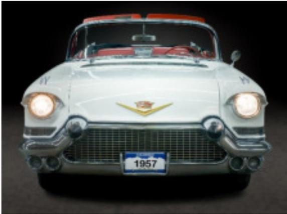
Eldorados sport dual circular headlights with chrome-lined eyebrows. Dual fins crown the front fenders, just aft of the headlights. The hood is lower than in previous years, devoid of top-side ornaments, and practically flush with the side fenders. Only a slight swale separates the hood and side fender.
