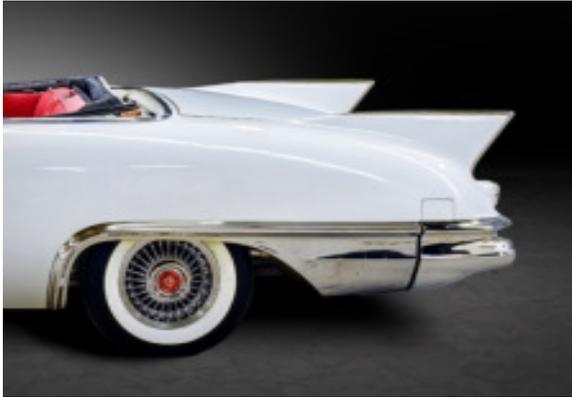
On the lower part of each rear fender is a stainless steel beauty panel that wraps around the rear corner and houses a round back-up light and exhaust port, each set into elegant rimmed receptacles. Topping this beauty panel is a broad, sculpted ridge that sweeps from the front of the rear wheel well, up and along the top of the wheel well, joining the top of the beauty panel, and following it all the way around to the rear.
