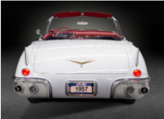
At the base of the fins are single, round taillights topped with chrome eyebrows, reminiscent of the headlights. These lights are combination brake, turn-signal, and running lights.
