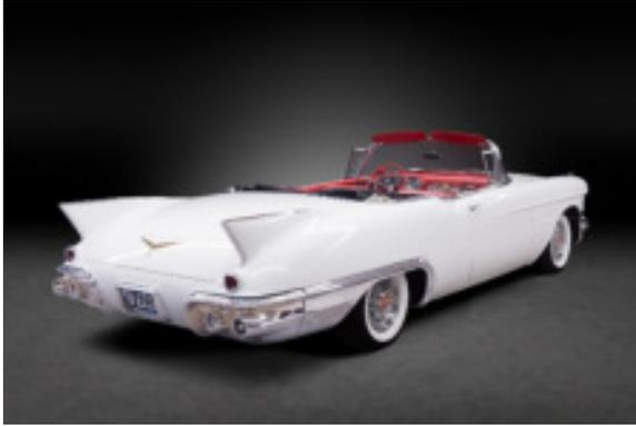
Back-swept shark fins sit inboard from the outside bulge of the rear fenders. These “stabilizer” fins are flat and horizontal along the top and pointed to the rear, while the back deck slopes downward. The overall effect is an illusion of blurring speed. Outlining these fins are simple chrome caps. The rear bumpers continue around the corner and match up with chrome molding over the wheel wells.
