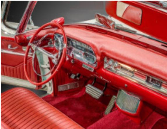
Cadillac worked hard to make the driver feel comfortable and in control. A matching-color steering wheel features a chrome inner horn ring. Gauges are limited to gas, speed, and water temperature, with warning lights for the parking brake and other issues. Easy-to-reach switches let the driver raise and lower windows, raise and lower the roof, open the trunk, and wash the windshield. Lighting includes an automatic map light, a lighted glove compartment, and even a lighted ashtray.
