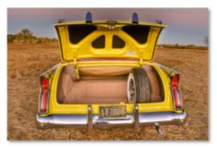
Despite the plunging trunk line, space inside the trunk is generous enough for a vertically mounted spare tire.
