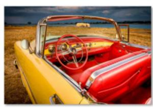
New for 1954 was the dramatic wrap-around windshield. The face of the dash continued the exterior color, sandwiched between a cap and base of the interior color.
