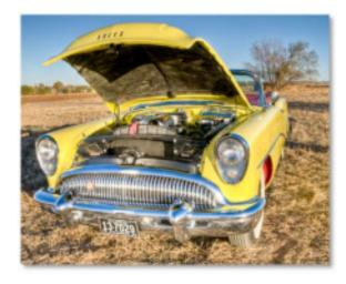
Cylinders were oversquare, meaning that the bore was larger than the stroke, 4.0 by 3.2 inches respectively. Valves were arranged in a straight line along each bank of cylinders, resulting in the term nailhead. This arrangement of valves and the increased compression ratio required a shaped crown for the pistons. Buick called them Power-Head Pistons.
