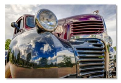
Curves, curves, curves dominate the front. Also visible is the sealed-beam headlight, which became standard in 1940.
