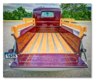
The bed consists of wood planks separated by steel skidstraps that prevent excessive wear of the wood. Wood beds continued in the Dodge line until 1985.
