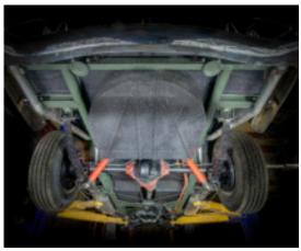
The rear suspension consisted of a live rear axle with longitudinal semi-elliptic springs and telescopic shock absorbers.
