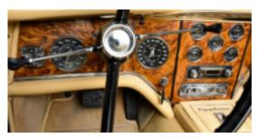
The dash has a tachometer, speedometer, low-fuel and turn-signal indicators, and the push-button selector for the automatic transmission.
