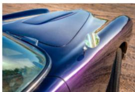
Though of limited production, The Vega's steel body panels were pressed rather than hand formed.
