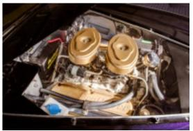
The 354 cubic inch (5.8 liter) engine turns out 325 horsepower and 425 foot-pounds of torque—unheard of in a European luxury car of the 1950s.
