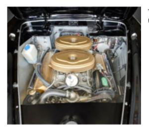
Twin air cleaners top the two 4-barrel Carter carburetors that feed the Chrysler Firepower Hemi engine.
