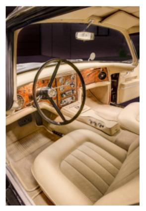
The interior is sumptuous and functional. The dashboard (fascia) of the Vega resembles that of an advanced aircraft. Large, legible gauges fill the space in front of the driver. Buttons and knobs spill off the dash and onto the console, putting controls ready to hand. The Facel Vega was among the first vehicles to sport a center console and a recessed steering wheel. A map light on a stalk is just another luxury feature. Bucket seats provide a balance of support and comfort.
