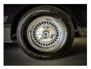
At the corners are Imperial wire wheels shod with Michelin P205/75R15, ensure that the two-ton vehicle can corner and stop as well as it can accelerate.
