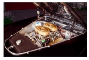
The engine compartment reveals what sets the Typhoon apart—a Chrysler Hemi engine—354 CID, producing 325 horsepower with PowerFlight transmission This view also shows the under-hood lights, quite the innovation in 1958.
