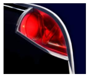
The innovative tail-light assembly shines light in 3 directions. A rear-facing bulb illuminates a translucent red fin embossed with the letter V. The stainless trim over the light preserved the flowing lines of the sill and fenders. All the stainless-steel trim benefitted from Facel's experience manufacturing office furniture.
