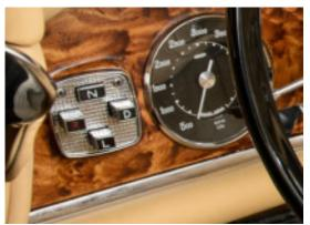
Along with the transmission, Facel employed the pushbutton selector with buttons for Neutral, Drive, Low, and Reverse, *but not* Park.
