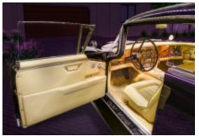
Careful design extends to even the door panels, which include a stainless grab handle, a vent-window winder, and switch for the electric window. Integrated into each door is a storage box with a lid.
