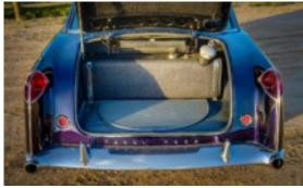
Facel preserved the integrity of the Vega's styling by locating the quick-release gas filter cap inside the trunk. Stainless trim extends to even the spare-tire cover.
