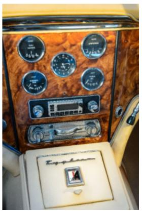
In the dash, above the center console, is an instrument cluster with a clock in the center, surrounded by gauges for water temperature, battery charging, gas level, and oil pressure. Below the cluster is an aftermarket stereo. And just below that are levers for heat and air.
