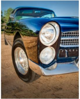
The front corners feature headlights on top and auxiliary lights on the bottom. Both are recessed in reflective coves.
